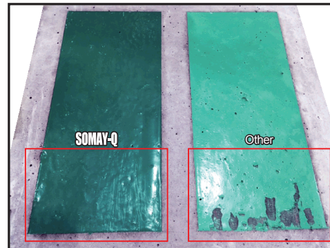
4Ever Concrete Floor Paint was painted over an oil-soaked substrate. Then a screwdriver was used to try to scratch off the coating. The competitor's coating delaminated easily. 4Ever Concrete Floor Paint did not delaminate whatsoever.
